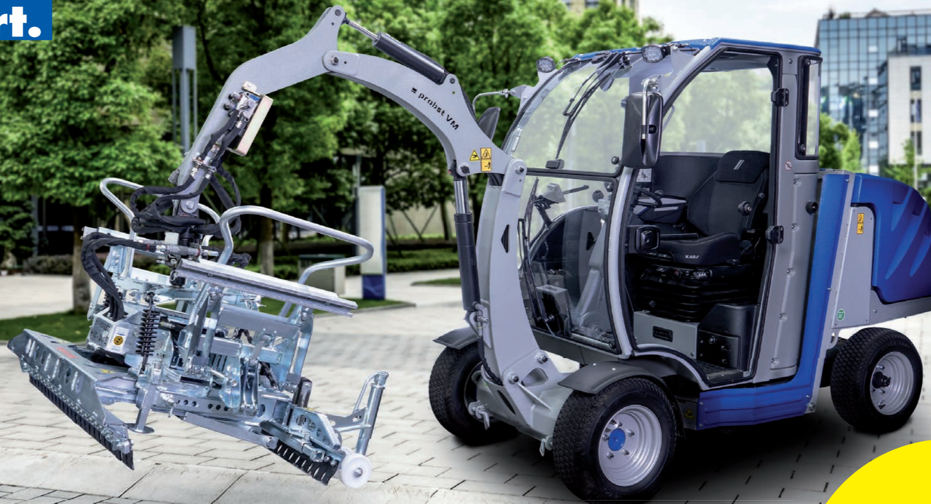
Paving machine VM-X-PAVERMAX premium with laying clamp HVZ-UNI-II
