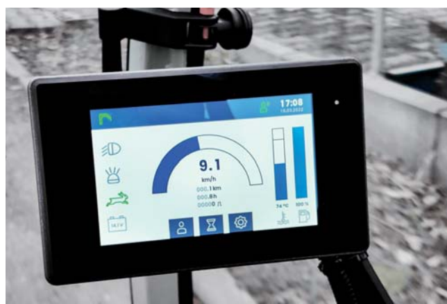
Colour LCD LED touch screen with display of real-time data and for selecting automatic programmes, driving profiles, ...
