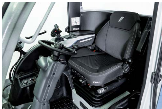
Decoupled driver's cabin with air-suspended comfort seat, seat heating and longitudinal damping
